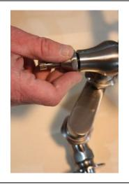
When using a wrench, we strongly advise not to have metal against metal as it could damage the surface of the part.
