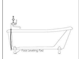
Use Velcro supplied to attach the claw feet to the floor.
