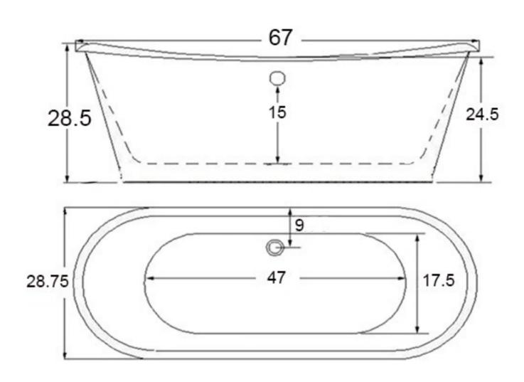
Tub weight empty 179 lbs Gallons to overflow 72 MA code Accepted UL Listed
