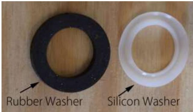
a black one that can be used if the drain hub is not perfectly square after installation. The black washer is designed to compress a little to compensate for an off square fitted drain hub. This washer should however be used for small mis-alignments only, we would strongly recommend that the 1.5" drain floor pipe be re-fitted if it is badly off square.
